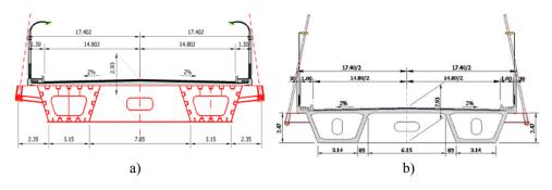
Fig. 9. Cable-stayed bridge superstructure. Cross-section: *a)composite deck; b)pre-stressed concrete deck*
