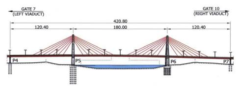
Fig. 2. Elevation of the main bridge in accordance with the initial solution
