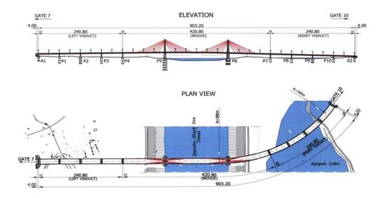
Fig. 1. Elevation and plan view of the bridge in accordance with the initial solution
