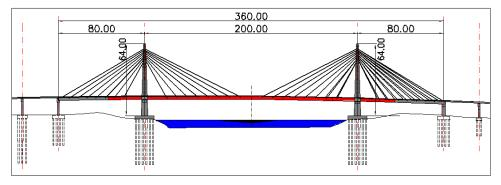
Fig. 4. Elevation of the main bridge in accordance with the changed solution
