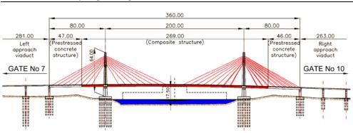
Fig. 8. Elevation of the main bridge in the proposed solution
