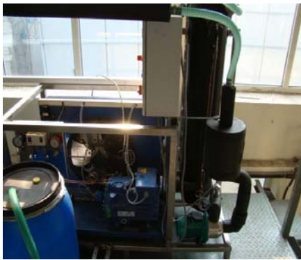
Fig. 10. Ice-slurry scraper-type generator
