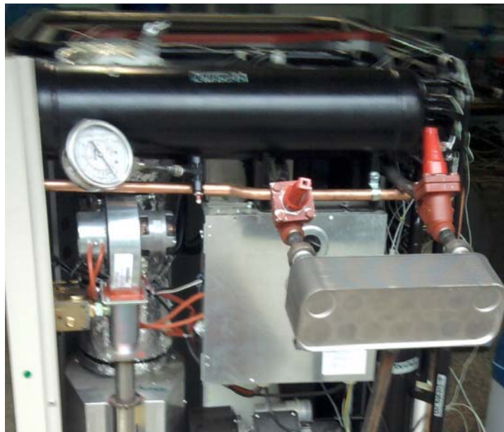
Fig. 6. ROBUR type absorption refrigerating systems using ammonia-water solution and modified vapor generator
